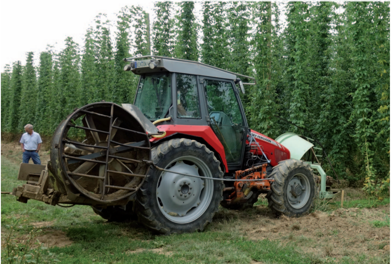
Mechanical hop stripping and suckering with a leaf vacuum cleaner
